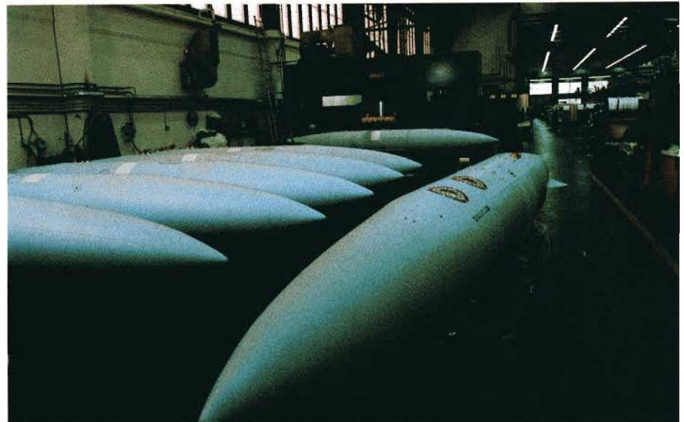
Fuel tanks for advanced aircrafts – F-16, produced by Nordisk Aluminium.
