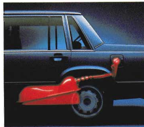
Plastics fuel tank system for the automotive industry.
